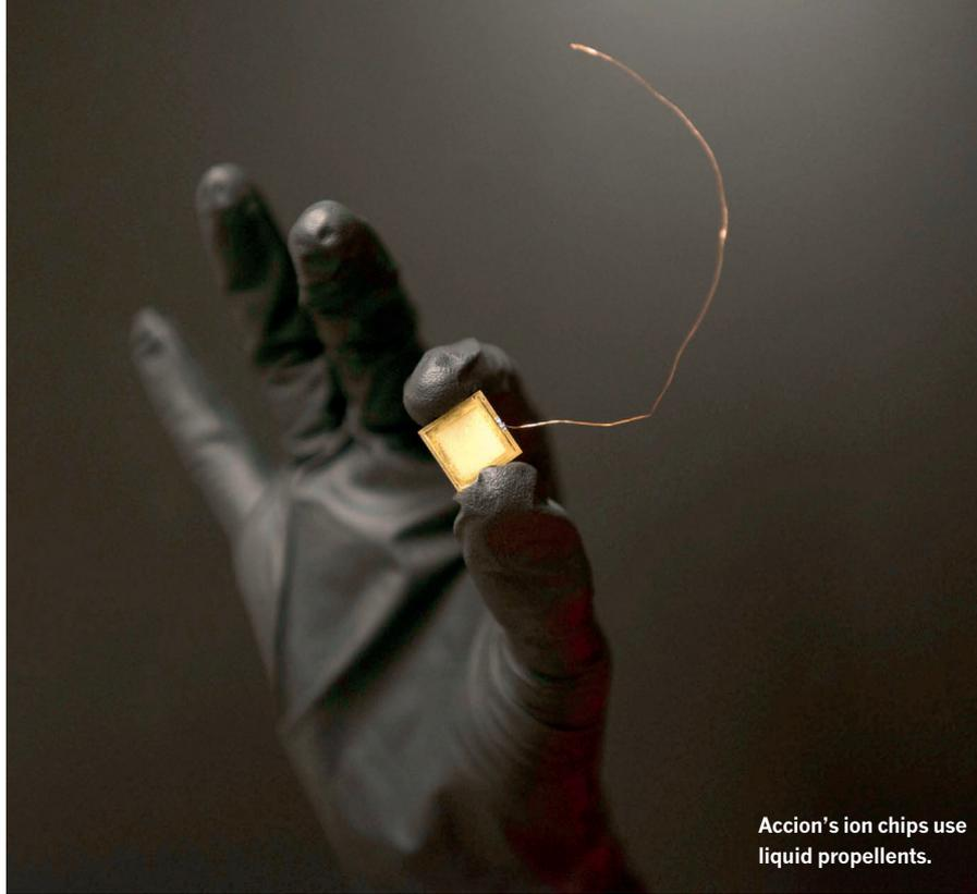
Accion's ion chips use liquid propellents.
